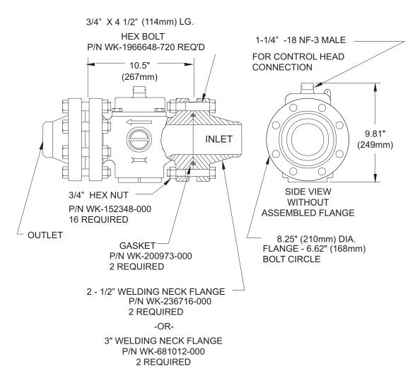
**Note:** Install valve with arrow pointing in direction of flow.
